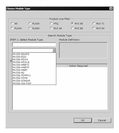
3 In the Product Line Filter area of the dialog box, select MVI56. In the Select Module Type dropdown list, select MVI56-PDPS, and then click OK to save your settings and return to the ProSoft Configuration Builder window.
