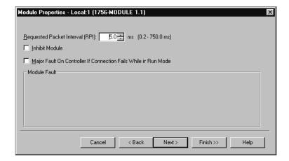
Select the Request Packet Interval value for scanning the I/O on the module. This value represents the minimum frequency the module will handle scheduled events. This value should not be set to less than 1 millisecond. Values between 1 and 10 milliseconds should work with most applications.
