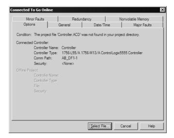
5 On the Connected To Go Online dialog box, click the General tab. This tab shows information about the processor, including the Revision (firmware) version. In the following illustration, the firmware version is 11.32
