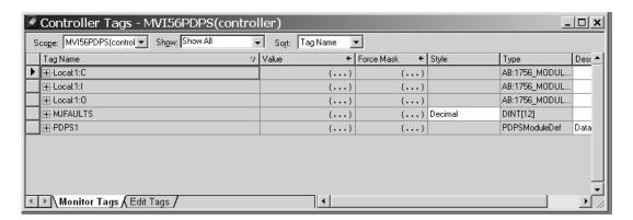
At this point, take the time to adjust the array sizes PDPS data table for the read and write data. The last step is to add the ladder logic. If you are using the example ladder logic, adjust the ladder to fit your application. If you are not using the ladder example, copy the ladder logic shown in the Controller Organization list shown to your application.
