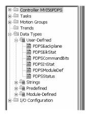
The next step in module setup is to define the data to be used to interface with the module and the ladder logic. Open the Controller Tags Edit Tags dialog box and enter the values shown in the following example. The MVI56-PDPS module is defined in the example as PDPS. You can set the tag name to any valid tag name you desire. If you are using the example ladder logic, this step has already been performed.
