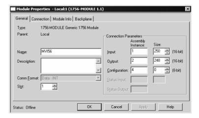
In the **Slot**: field, use the spinners on the right side of the field to select the slot number where the module will reside in the rack, and then click OK.
