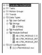
The next step in the module's setup is to define the User Defined Data Types to be used with the module. Copy these data types from the example ladder logic if you are not using the example. They will be defined if you are starting from the example ladder logic. The Controller Organization list should display the User Defined Data Types shown in the following example:
