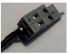
3 Insert the connector into the power port on the bottom of the ICX30-HWC.
