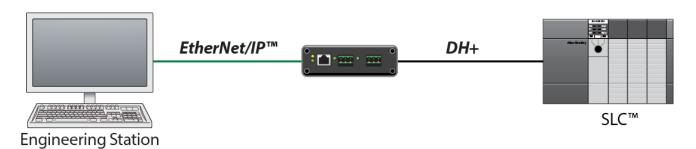
This mode acts as a bridge between an EtherNet/IP and a Data Highway Plus network.
