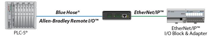
This mode allows PLC's on Remote I/O to connect to and control 1794-AENT EtherNet/IP Flex adapters.
