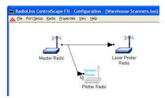
To remove a RF link between two radios, select the line between the radios.
