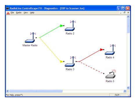
The colored lines indicate the signal strength of each radio, see Viewing Signal Strength. If any of the communication links show red dashed lines see Broken Links in a Radio Network (page 68).
