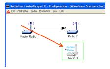
Continue on to Graphically Define the RF Link (page 38) to define the communication links between radios.
