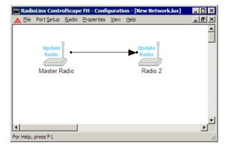
Double-click the left mouse button on the Master Radio to open the Radio Properties dialog box.
