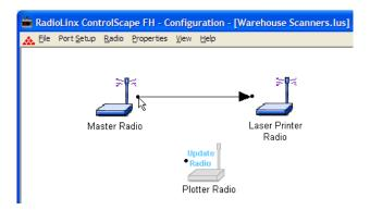
Hold the left mouse button down and drag the RF link to the Remote radio's link point (located to the left of the Remote radio). As the mouse is being dragged, a line will appear between the Master and Remote radios. **This is the graphical representation of the RF communication link.** After the mouse button is released an arrowhead will appear at the end of the graphical link line at the Remote radio's link point.
