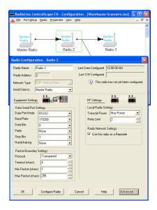
**Important:** The items on this dialog box depend on what type of radio you select. The example in this topic shows a RadioLinx IFHS (Industrial Frequency Hopping Serial) radio. Refer to the user manual for your radio for an explanation of each configuration item.
