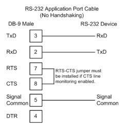
**Note:** If the serial device is configured with to use the CTS line, then a jumper is required between the RTS and the CTS line on the radio connection.
