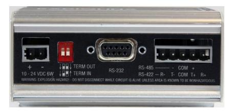
The application ports are located on the bottom of the radio. Do not use the "CONFIG" port on the top of the radio to connect your device network.
