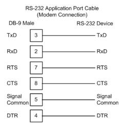
The "Use CTS Line" parameter for the serial device should be set to 'Yes' for most modem applications.
