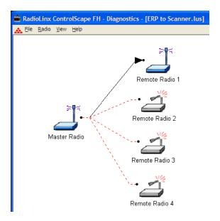
One of the most common reasons radios do not communicate is an incorrect setting in the "Send Data To" field in the Radio Configuration dialog box. Verify that the radio is sending to and receiving from the correct radio ID.
