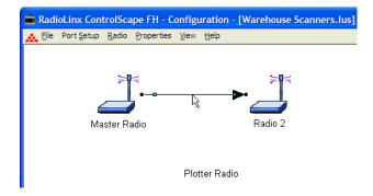
Press the Delete key to remove the graphical link line between the radios. Now a repeater could be added between the two radios or the radios could be connected to other radios.
