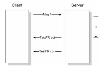
If the module does not receive the TESTFR.con message within a certain amount of time, it will timeout and close the connection. You can configure the timeout period using the following parameter:
