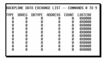
**Tip:** Repeat this command at one-second intervals to determine the number of blocks transferred each second.
